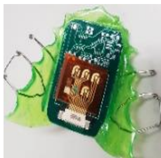
Figure 1: a) Device for continuous monitoring of health parameters within the oral cavity. b) Potentiometric measurement of pH. Shown are measurements with phosphate buffers of the indicated pHs and measurements with three different saliva samples. (b) Amperometric response of glucose sensors.
