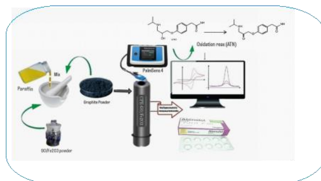
Figure 1: Schematic determination of ATN with Fe 2 O 3 -rGO/CPE sensor
