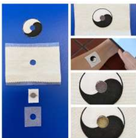
Figure 1: Wax screen-printed fabric-based colorimetric microfluidic device.
