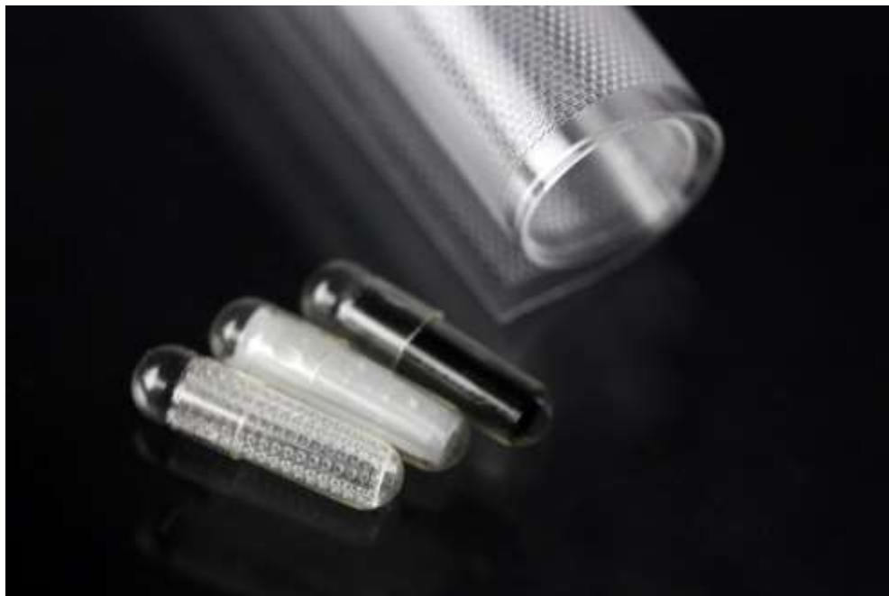
Figure 1: Example of microdevice for oral drug delivery. This is a self-unfolding foil that aligns to the intestinal wall (rat or pig). Hereby, we have, among others, achieved oral delivery of insulin [2]
