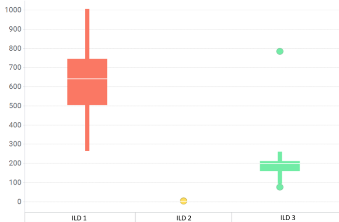
Figure 1: Defect level for different ILD materials after identical post CMP cleaning
