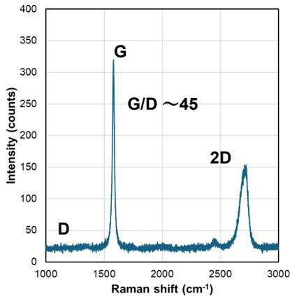
Fig. 4. Raman spectrum after CVD. Highly crystalline MLG was deposited.
