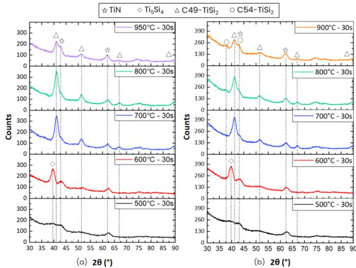
**Figure 3.** Grazing incidence X-Ray patterns corresponding to the evolution of the Ti/Si:P system as a function of different rapid thermal annealing temperatures, 30 s annealed in an N<sub>2</sub> atmosphere for (a) low-doped and (b) high-doped Si:P epitaxial layers.
