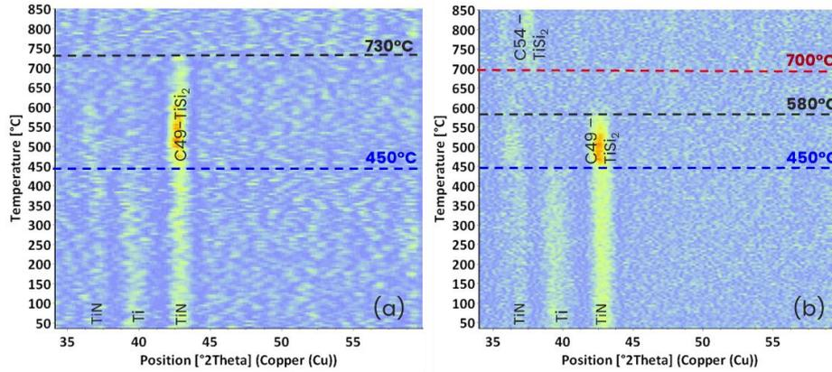
**Figure 1.** *In-situ* X-ray diffraction mappings corresponding to the reaction between a 10 nm Ti metal layer deposited on (a) low-doped and (b) high-doped Si:P (100) epitaxial layers. The blue dashed lines correspond to the temperature of full metal consumption and the C49 TiSi<sub>2</sub> identification. The black lines correspond to the C49 phase disappearance and the red lines to the growth of the C54 phase.
