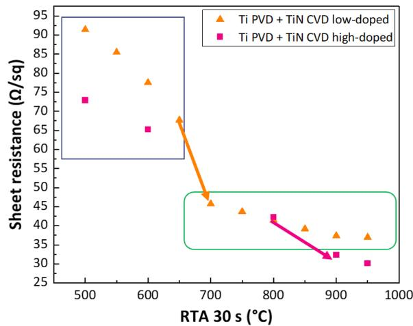
**Figure 2.** Evolution of the sheet resistance  $R_s$  for different rapid thermal annealing temperatures in the Ti/Si:P system with high-doped (pink squares) and low-doped (orange triangles) Si:P epitaxial layers. Samples were annealed for 30 s in an N<sub>2</sub> atmosphere.
