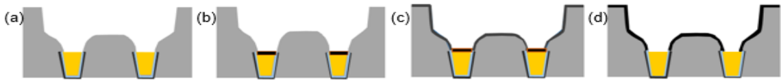
Fig. 1. Process sequence of selective ALD TaN Deposition (a) after pre-clean for interface (b) SAM deposition (c) selective ALD TaN deposition (d) SAM removal process
