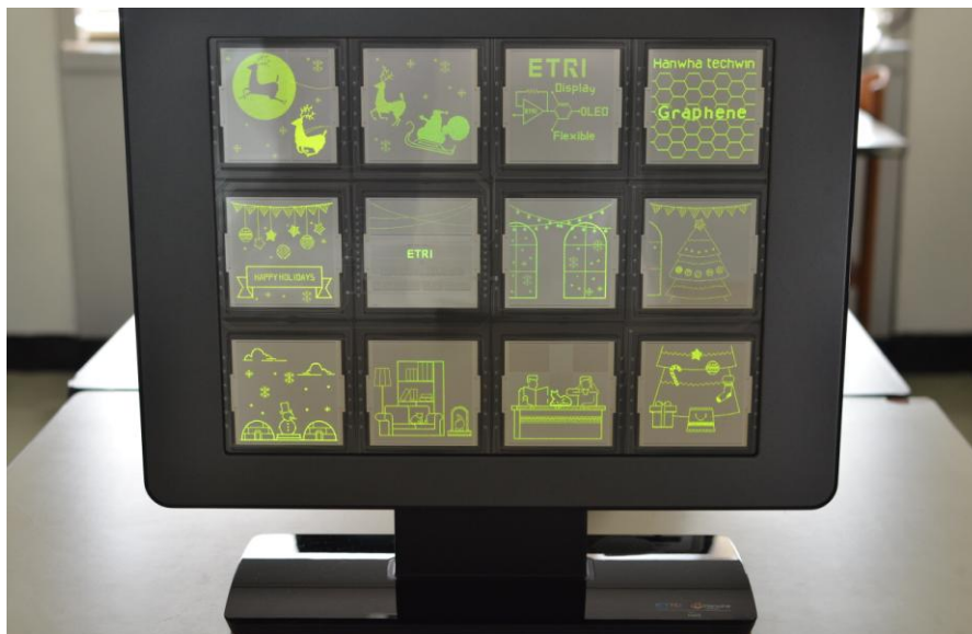
Figure 1: Gen 2 (370 mmx470 mm) sized Graphene anode OLED
