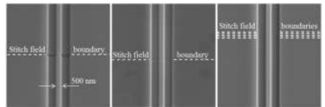
Figure 2: Etch effect milling artifacts at stitch field boundaries: a) if no further strategies are
