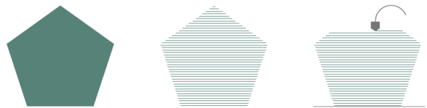
Figure 1: FFF part printing process including geometry definition, CAD slicing and material extrusion.
