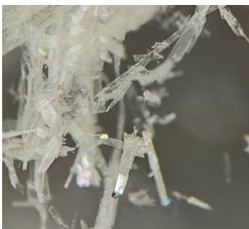
Figure 1: Microscope Image of Orthorhombic Crystals structures of MoO 3 ( \alpha -MoO 3 )
