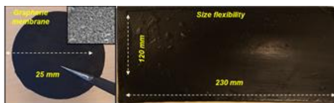
Figure 1: 3D-printed graphene-based membranes with various sizes. SEM image confirms the porous nature of the 3D-printed membrane.
