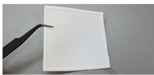
Figure 2: DLP 3D printed membrane (RIC2D group proprietary picture)
