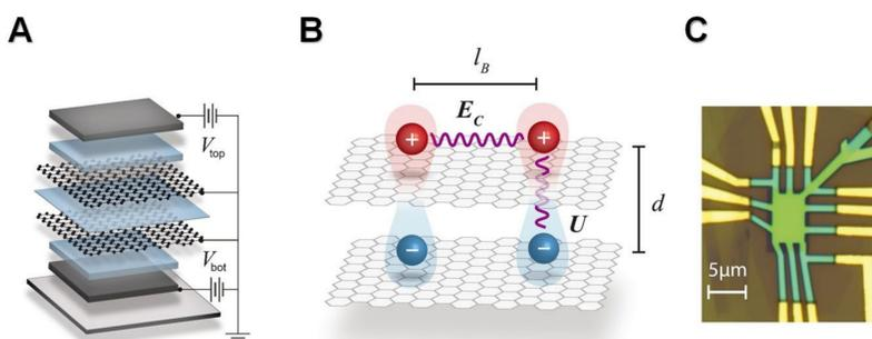
**Fig.1** (A) Van de Waals Heterostructure for the device. (B) Illustration of the energy and length scales associated with exciton pairing in a graphene double-layer structure under a magnetic field. (C) Optical image of a graphene double-layer device used in this study.
