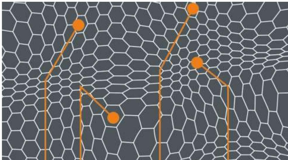
**Figure 1:** Schematic representation of what corrugations and strain fluctuation might look like in graphene.
