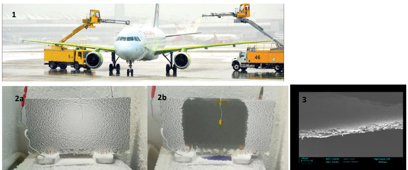
Figure 1: Typical de-icing process of an airplane through propylene glycol spray
