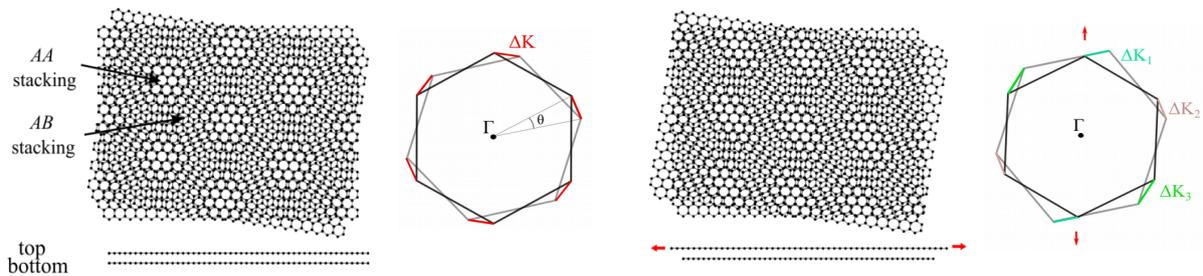
**Figure 1:** Sketch of a TBLG with (left) and without (right) heterostrain, with their respective Brillouin zones. The stress is applied to the top (grey) layer as represented by the red arrows.
