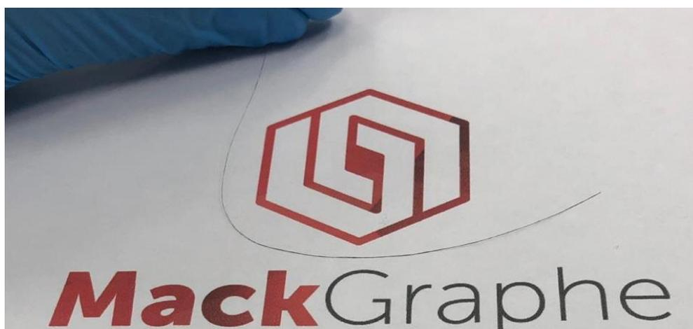
**Figure 1:** Graphene oxide fiber prepared by the microfluidic device.
