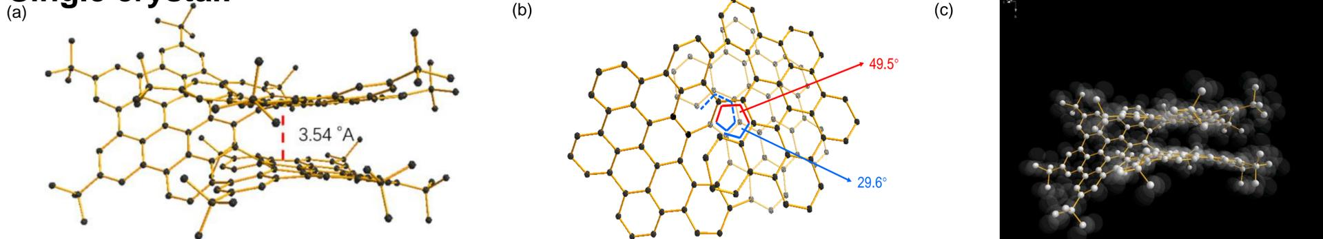
Crystal structure of **NHBNG 1** (a) side view, (b) top view of the  $\pi$ -extended helical geometry of **NHBNG 1**, as well as torsion angles of the embedded heptagon unit (The hydrogen atoms and tert-butyl groups are omitted for clarity). (c) video of the single crystal
