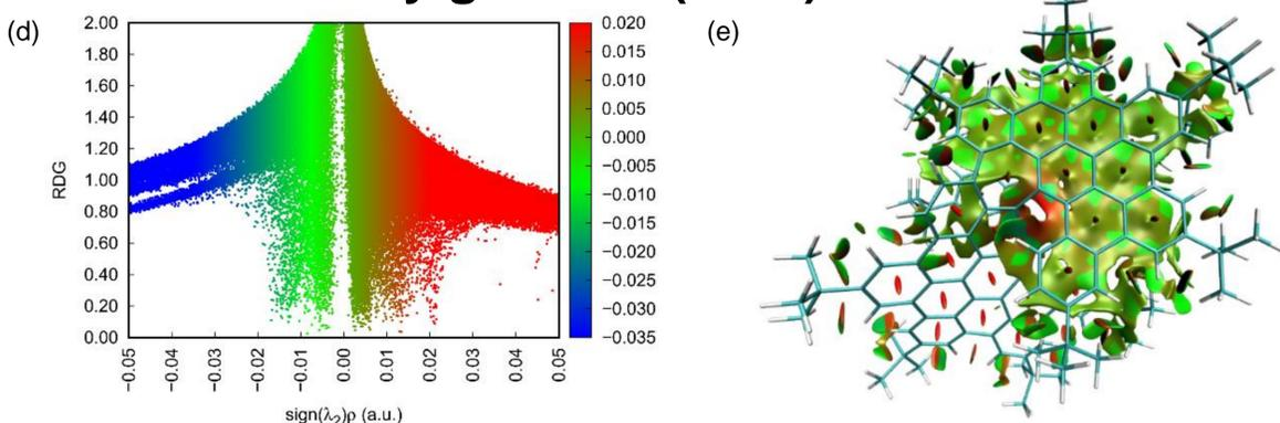
(d) Graphical representation of the reduced density gradient (RDG) versus  $\text{sign}(\lambda_2)\rho$ , in which the blue, green, and red color of the vertical scale represent the hydrogen bonding, Van der Waals effect and steric effect, respectively. (e) Plots of the reduced density gradient isosurfaces for compound **NHBNG 1**.
