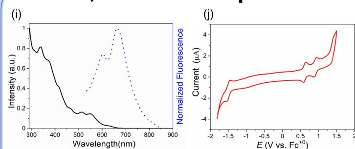
(i) UV-vis absorption (black line) and photoluminescence emission (PL, dashed blue line, excitation at 510nm) spectra of **NHBNG 1** in  $\text{CH}_2\text{Cl}_2$  ( $1 \times 10^{-5} \text{ mol/L}$ ). (j) Cyclic voltammetry (CV) of **c** in  $\text{CH}_2\text{Cl}_2$  containing  $0.1 \text{ M } n\text{Bu}_4\text{NPF}_6$  at a scan rate of  $50 \text{ mVs}^{-1}$  at room temperature.
