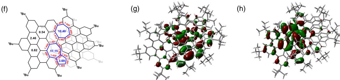
(f) Nucleus independent chemical shift calculations (NICS(1)) values (blue/black) of **NHBNG 1**, calculated at the GIAO-B3LYP/6-31+G(2d,p) level of theory, as well as the bond lengths (red, in  $\text{Å}$ ) of the embedded heptagon-azulene units. Frontier molecular orbitals of **NHBNG 1** (g) HOMO (h) LUMO. The calculations were performed at the B3LYP 6-31G (d) level.
