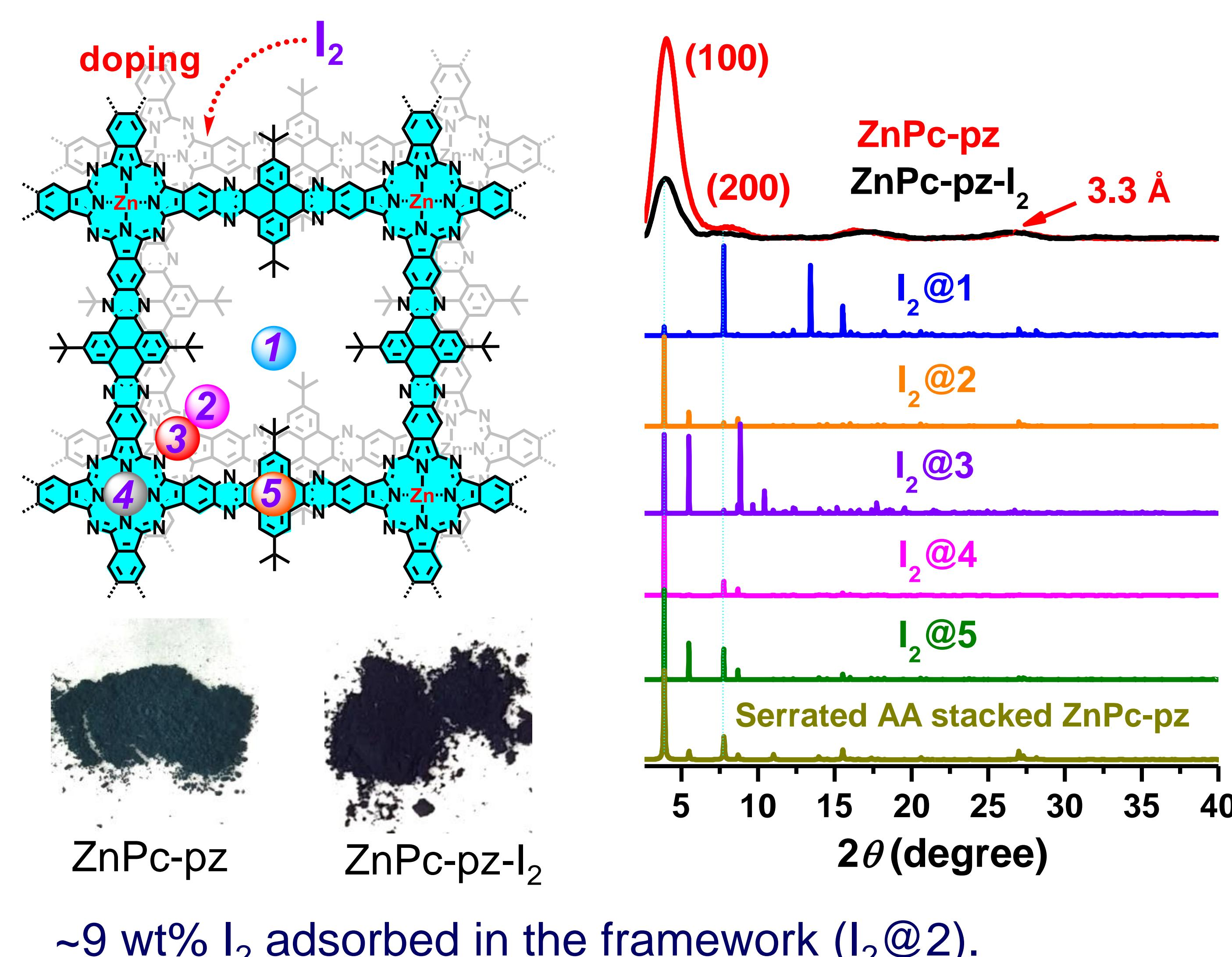
~9 wt% I<sub>2</sub> adsorbed in the framework (I<sub>2</sub>@2).
