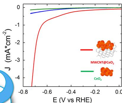
LSV for MWCNT@CeO<sub>2</sub> (red line), the bare GC electrode (blue line) and CeO<sub>2</sub> NPs (green line) in a CO<sub>2</sub>-saturated solution. Scan rate: 2 mV s<sup>-1</sup> in HNO<sub>3</sub> 0.1 M.
