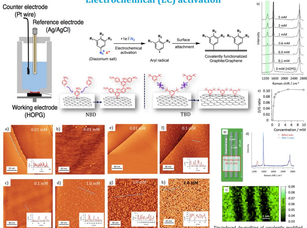
Concentration dependent covalent modification of graphite using diazonium chemistry. (a-d) NBD and (e-h) TBD. It can be readily noticed from this STM data that efficiency of covalent modification is superior for TBD
