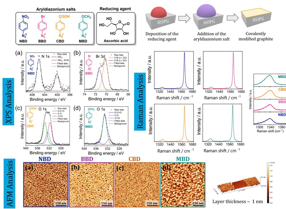
Ascorbic acid mediated diazonium chemistry provides a fast, simple and efficient way of covalent functionalization of HOPG where the highly dense covalent monolayers with thickness less than 1 nm could be formed from a number of different diazonium salts.
