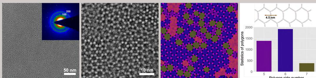
120 kV TEM overview image 120 kV AC-HRTEM image. Analysis of the distribution of hte polygons in the AC-HRTEM by a neural network of U-net architecture.
