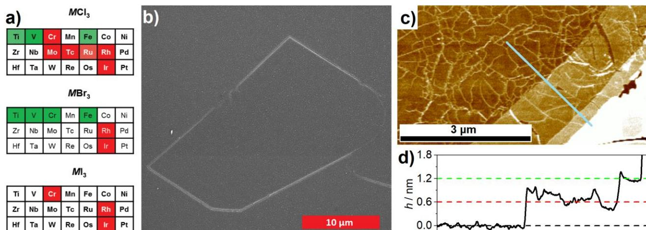
**Figure 1:** a) overview of transition metal trihalides with 2D structure (red:  $\text{AlCl}_3$ -type, green:  $\text{BiI}_3$ -type) [1], b) SEM image of an as grown  $\text{Cr}_x\text{Ru}_{1-x}\text{Cl}_3$  nanocrystal with a height of ca. 30 nm (surface particles and cracks can be attributed to carbon sputtering), c) AFM image of a  $\text{Cr}_x\text{Ru}_{1-x}\text{Cl}_3$  fewlayer structure obtained by delamination, d) height profile of the in c) shown step of a mono- and bilayer.
