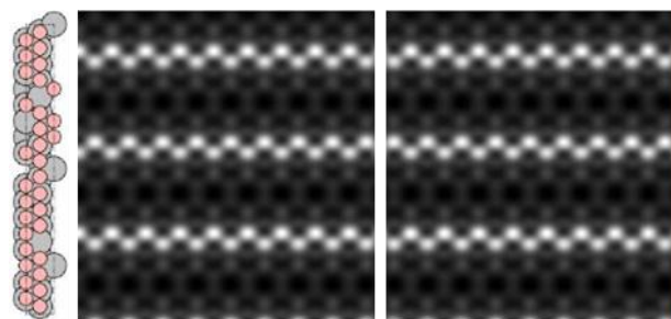
Figure 1. STM imaging of \beta 8 borophene allotrope on an Ag substrate. 3D structure (left) with B and Ag atoms in pink and grey, respectively. STM image simulation from DFT calculations (center) and the Unet-Tool (right).
