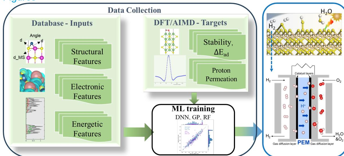
Figure 1. Schematic illustration of discovery materials for HER catalysts and PEMs.
