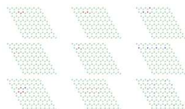
Figure 2. Examples of stable configurations found inside different classes with 4, 9, and 14 defects. Larger points for middle layer atoms; smaller pairs for outer layers. Green shows defect-free areas, red for vacancies, and purple for substitutions.
