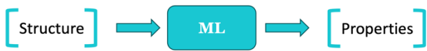
Figure 2. Crystal structure to materials properties prediction model for high throughput screening of an enumerable space of crystal structures in a Wyckoff position representation. The model crawls the space of all possible structures as inputs and predicts the materials properties.
