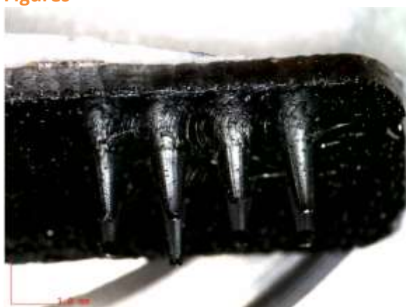
Figure 1. Graphene-based conductive coating on polymer microneedles
