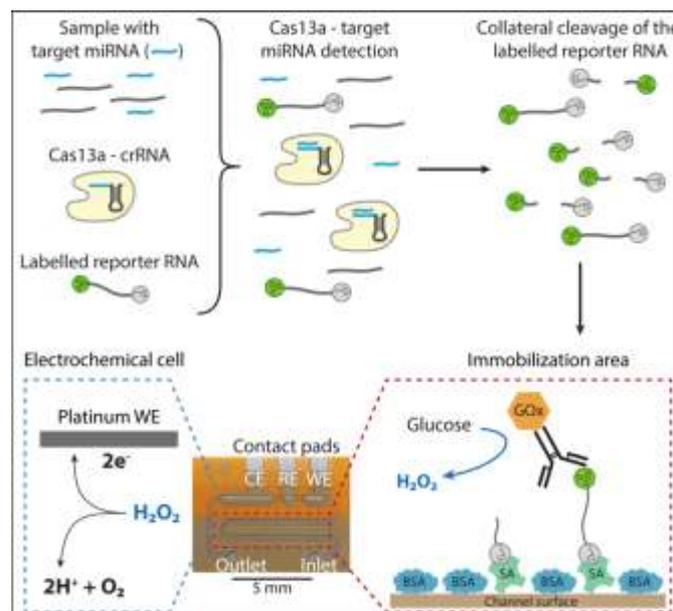
Figure 1. The working principle of the electrochemical CRISPR-Biosensor [4].
