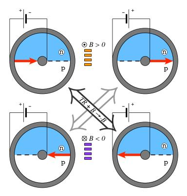
Figure 1. Quantum Hall states propagating along a p-n junction in the strong-field limit, for B > 0 (top) and B < 0 (bottom). Diagonal double arrows indicate the system symmetry upon a simultaneous time reversal and magnetic field inversion.
