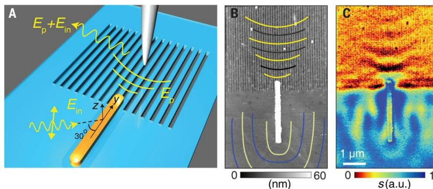
**Figure 1.** (A) Schematic of the experiment. (B) Topography image. The lines illustrate wavefronts of phonon polaritons on the hyperbolic metasurface (yellow and black) or phonon polaritons on the unpatterned flake (yellow and blue). (C) Near-field optical image. It clearly reveals concave wavefronts of phonon polaritons emerging from the rod's upper extremity.
