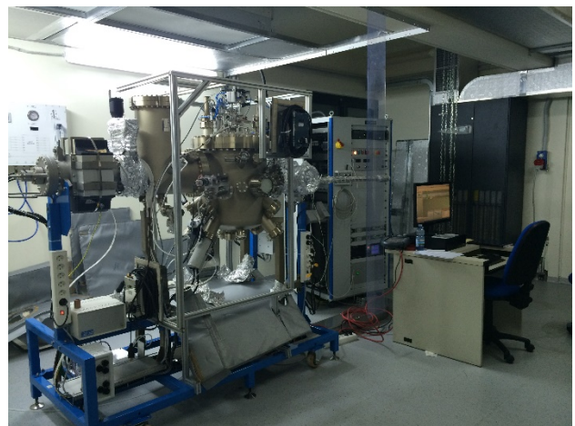
Figure 1. Photograph of the MBE facility installed at IMM-CNR in Lecce.
