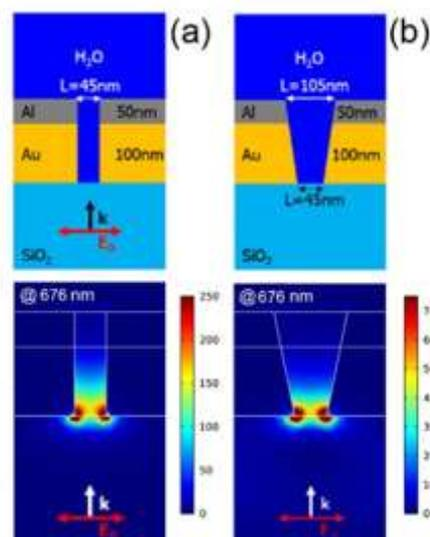
**Figure 2. Top:** ketch of a section of the ideal (a) and fabricated (b) rectangular Au-Al nanoslot. **Bottom:** near-field distributions of the ideal (a) and fabricated (b) Au-Al nanoslot at the experimental excitation wavelength (676 nm). The section planes of the rectangular antennas are parallel to the short axis.
