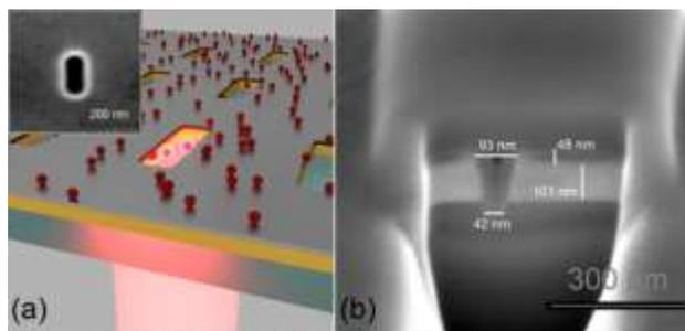
**Figure 1.** SEM images of the fabricated structures. (a) Schematic illustration of the Au-Al nanoslots; **Inset:** SEM micrograph of a fabricated nanoslot; (b) Au-Al nanoslot, cross section. A 101 nm gold layer and a 48 nm aluminum layer are visible. A platinum layer is visible on top, deposited to improve the cross section cut.
