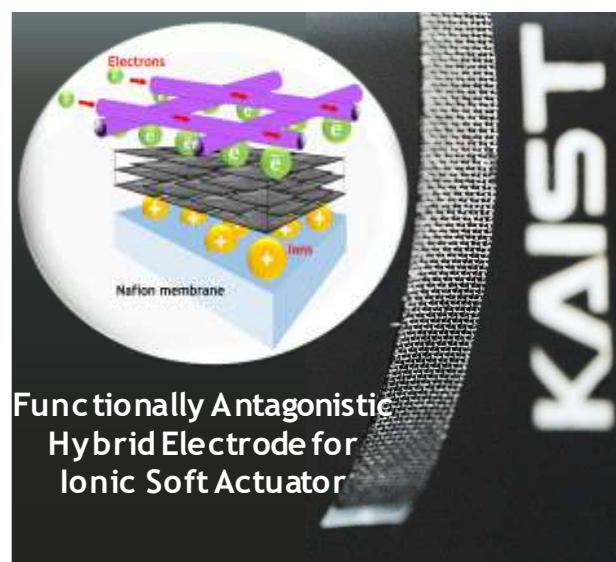
Figure 1. Functionally antagonistic hybrid electrode based on graphene mesh and nitrogen-doped graphene.
