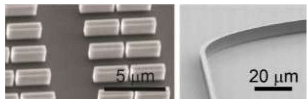
Figure 1. Scanning electron microscope images of Ge antennas supporting localized plasmon resonances (left) and of a Ge waveguide (right).
