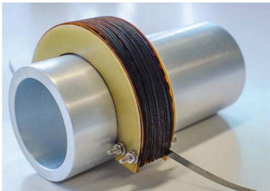
Prototype thermoelectric generator uses waste heat at the surface of pipes
