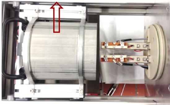
Stage 2: copper heating block embedded with heater and temperature control
