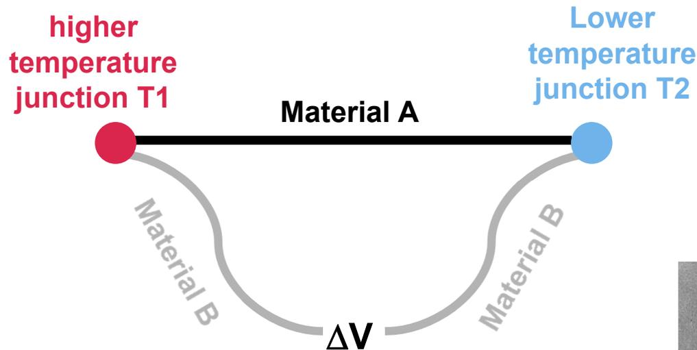
When the two junctions are kept at different temperatures, a thermovoltage is produced in the circuit.
