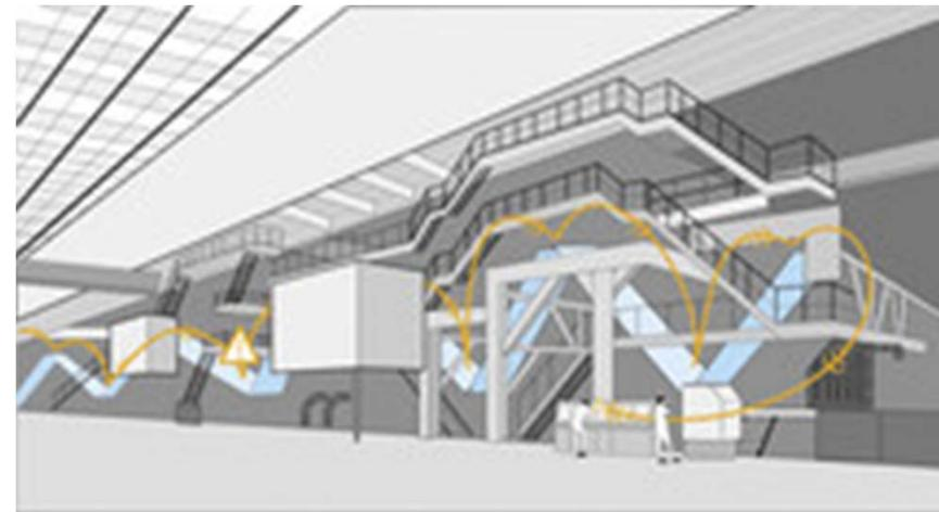
Example paper machine: heat generated by drying processes enables the use of sensors controlling the production process
