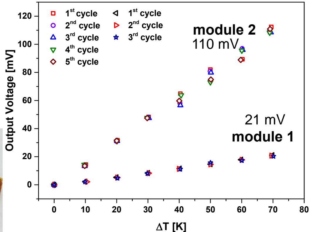
Planary type: TEG1 with 4 thermocouples (4 layers p-type & 4 layers n-type)
