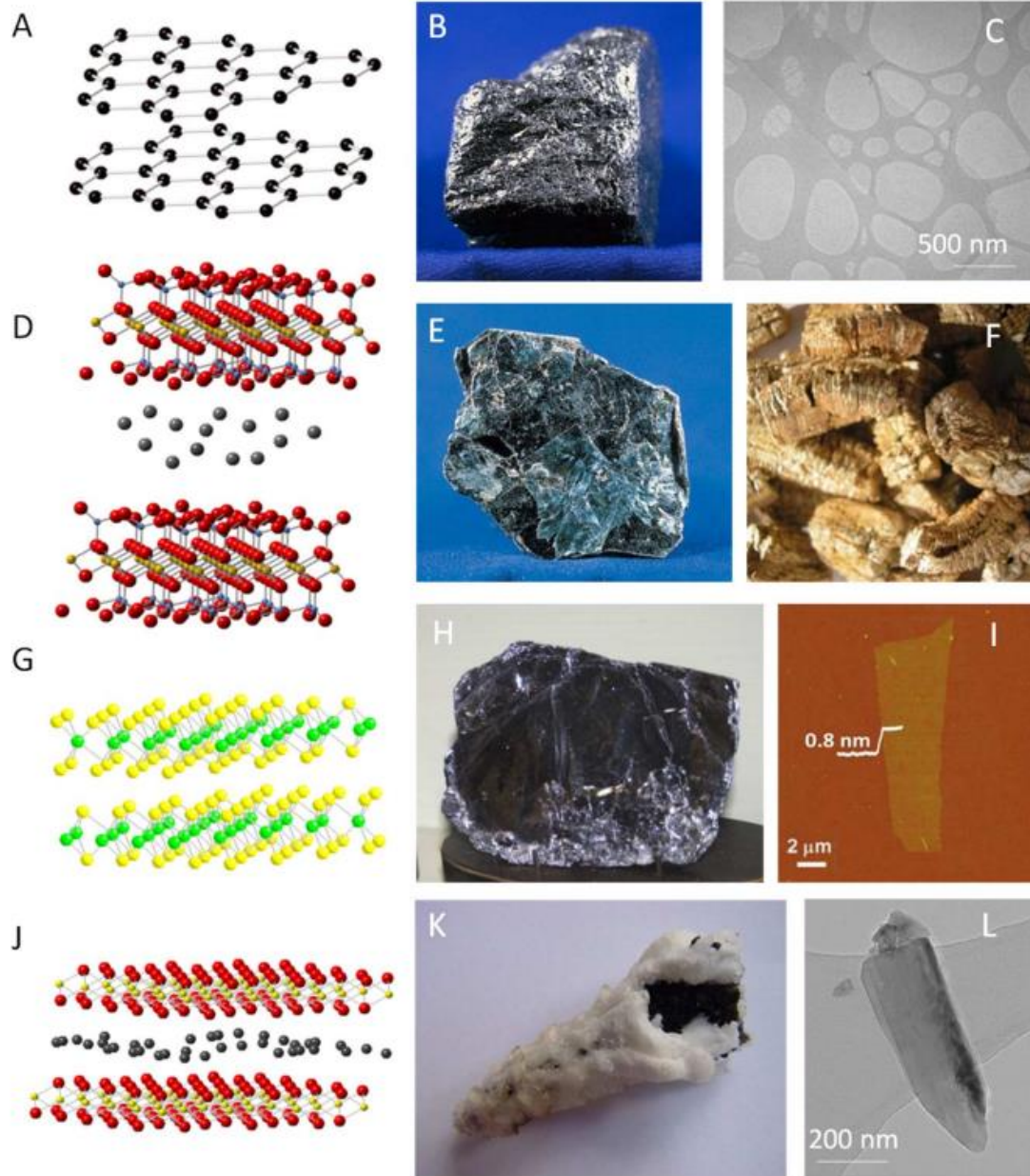
Fig. 1. Crystal structures, naturally occurring forms, and exfoliated products for four example layered materials. (A) Graphite consists of alternating stacks of hexagonally arranged carbon atoms (black spheres), (B) is a naturally occurring mineral, and (C) exfoliates to single atomic layers of carbon called graphene. (D) Vermiculite is a layered silicate hydrate (typically Mg_{1.8}Fe_{0.9}Al_{4.3}SiO_{10}(OH)_2 \cdot 4(H_2O) ) that (E) is found naturally as a mineral and (F) can be exfoliated, for example, upon heating. Silicon atoms are in blue, oxygen atoms are in red, Al/Mg/Fe atoms are in yellow, and interlayer counterions are in black (H and H_2O not shown). (G) MoS_2 is a layered arrangement of S and Mo atoms (chalcogen atoms are in yellow, and transition metal are in green) that (H) is found naturally as the mineral molybdenite and (I) can be exfoliated to MoS_2 monolayers. (J) Layered manganese dioxide (manganese atoms are in yellow, oxygen is in red, and interlayer counterions are in black) occurs naturally (K) as birnessite and (L) can be exfoliated to give MnO_2 nanosheets. (C), (I), and (L) are adapted from (48), (87), and (58), respectively. The layer spacings for each material are graphite, 0.35 nm; vermiculite, 1.5 nm; MoS_2 , 0.6 nm; and MnO_2 , 0.45 nm.
