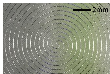
Figure 2. Printed antenna pattern on PLA substrate
