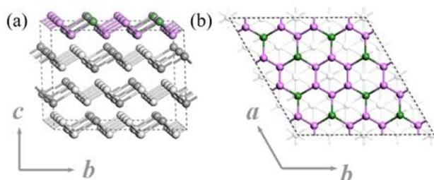
Figure 1. Structure of bulk  $\text{GeP}_3$  in a  $2 \times 2 \times 1$  supercell from side (a) and top (b) views. Pink and green balls represent P and Ge atoms, respectively.
