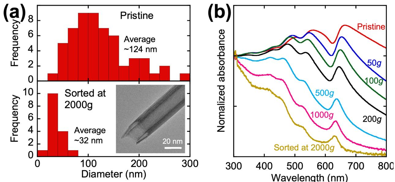
**Figure 1:** Sorting of inorganic nanotubes. (a) Diameter distribution of the pristine (top) and sorted WS<sub>2</sub> nanotubes (bottom). The inset represents a typical TEM image of the sorted WS<sub>2</sub> nanotubes. (b) Optical absorption spectra of the pristine and sorted WS<sub>2</sub> nanotubes.
