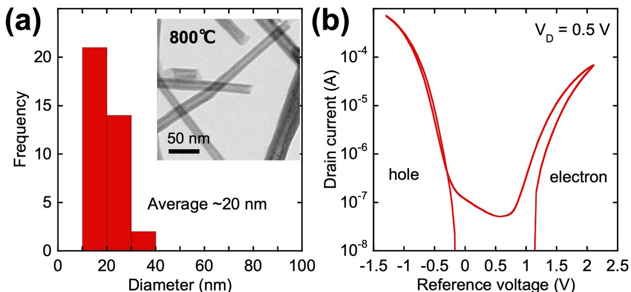
**Figure 2:** Synthesis of inorganic nanotubes. (a) Diameter distribution of the synthesized WS<sub>2</sub> nanotubes. The inset represents a typical TEM image of the synthesized WS<sub>2</sub> nanotubes. (b) Transistor characteristics of the network film of the synthesized WS<sub>2</sub> nanotubes.
