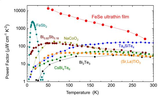
Figure 1: Temperature dependence of thermoelectric power factor in FeSe ultrathin film and typical thermoelectric materials.
