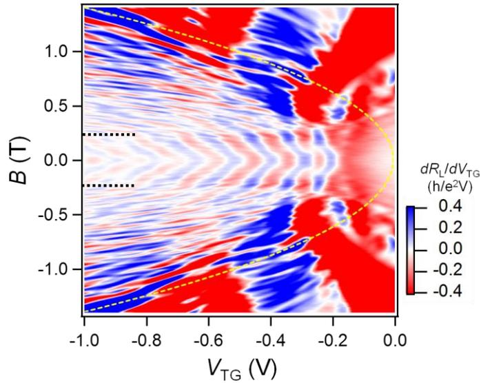
**Figure 1:** A  $B$ - $V_{TG}$  mapping of  $dR_L/dV_{TG}$  at  $V_{BG} = 1.2$  V and at 6 K in an hBN/graphene/hBN device with a QPC. Carrier density in whole graphene device was controlled by a back gate bias, and p-n junctions were formed by local control of carrier density by top split gates. Fabry-Pérot oscillations due to the interference in n-p-n cavities were observed at  $|B| < \sim 0.2$  T, and they collapsed under higher magnetic fields.
