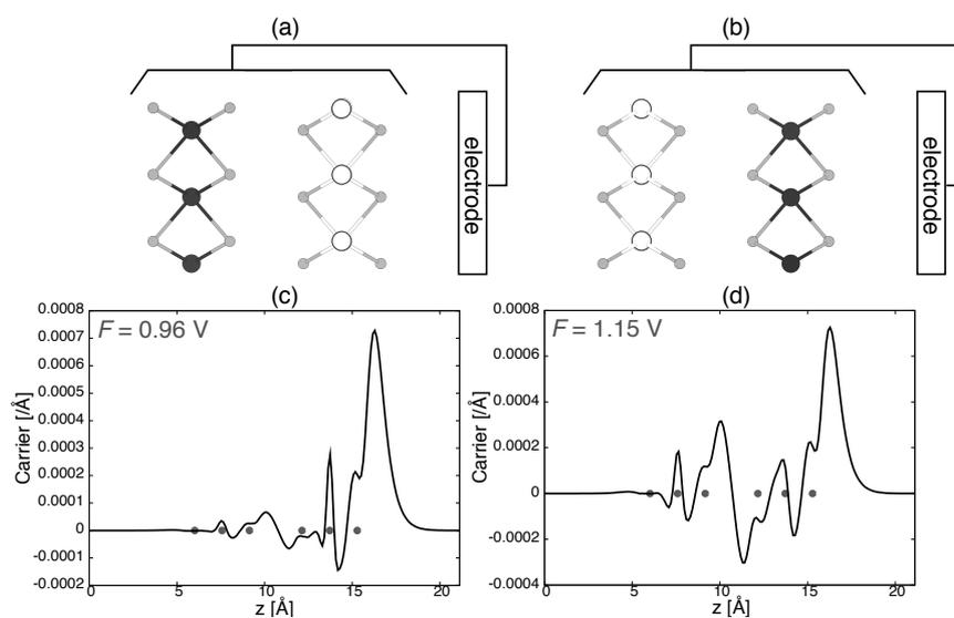
**Figure 1:** Structural models of (a) WS<sub>2</sub>/MoS<sub>2</sub>/electrode and (b) MoS<sub>2</sub>/WS<sub>2</sub>/electrode arrangements. White, gray, and black balls denote Mo, S, and W atoms, respectively. Carrier distribution in heterosheet of MoS<sub>2</sub>/WS<sub>2</sub> for (c) WS<sub>2</sub>/MoS<sub>2</sub>/electrode and (d) MoS<sub>2</sub>/WS<sub>2</sub>/electrode arrangements.
