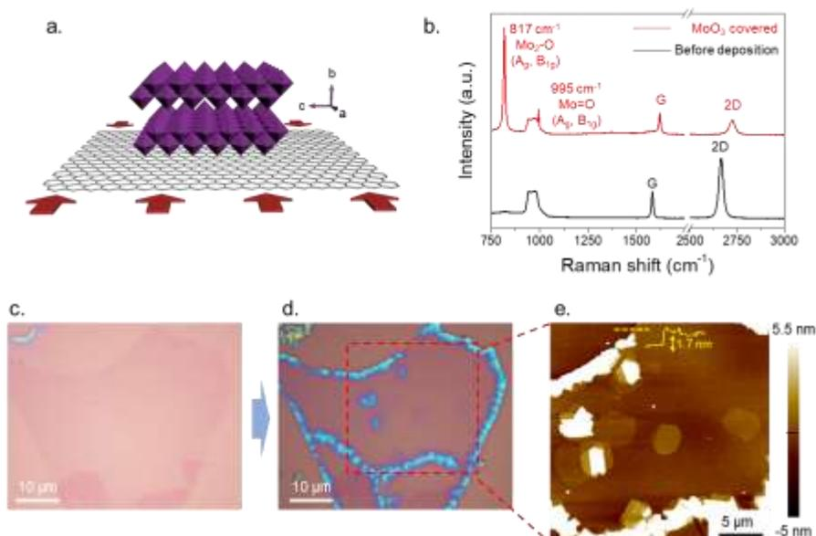
**Figure 1:** (a) Schematic image of graphene-MoO<sub>3</sub> heterostructure. (b) Raman spectra of pristine 1L graphene and graphene-MoO<sub>3</sub> heterostructure. (c, d) Optical microscope image of pristine graphene and graphene-MoO<sub>3</sub> heterostructure, respectively. (e) Atomic Force Microscope (AFM) image of graphene-MoO<sub>3</sub> heterostructure.
