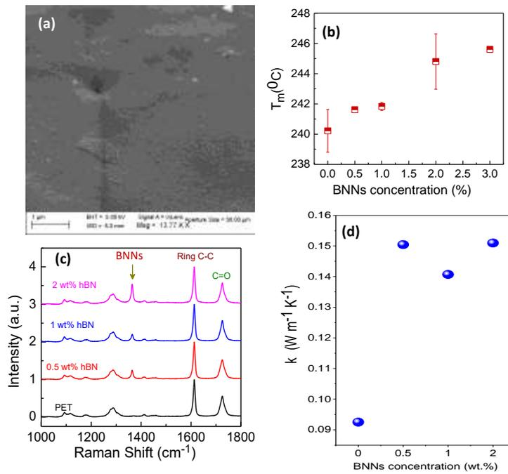
**Figure 1:** (a) Cross-sectional SEM image of a typical PET:BN composite film. (b) Increasing melting temperature of PET:BN composite as a function of BNNs filler concentration (wt.%). (c) Raman signatures for various PET:BN nanocomposite films. (d) Thermal conductivity as a function of BNNs filler concentration.
