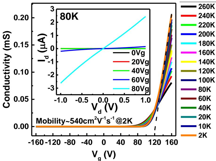
**Figure 2:** Evolution of conductivity versus gate-voltage curves for tri-layer InSe FET with varied temperatures. The inset plot shows the  $I_d$ - $V_d$  curves with different gate voltages at 80K.
