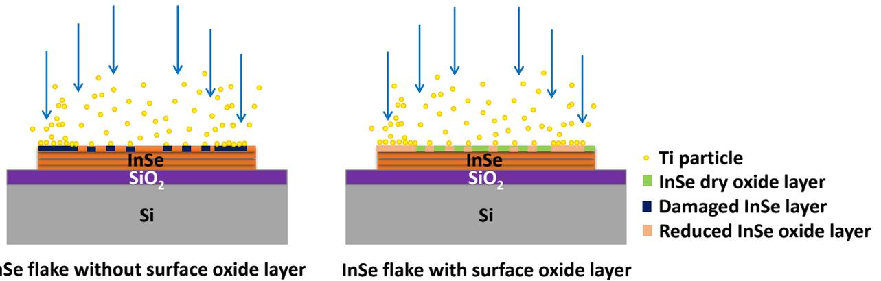
**Figure 1:** Schematic representation of indium selenide flakes with or without surface oxide layer. Titanium particles tend to react with InSe and damage it when there is no surface oxide layer. On the other hand, titanium particles will reduce the surface oxide layer of InSe instead if there exists an oxide layer.
