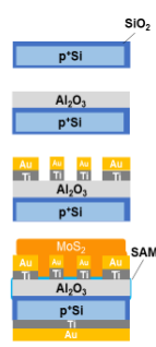
Figure 1: Fabrication process and device structure.
