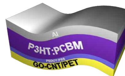
Anode in flexible OPV
